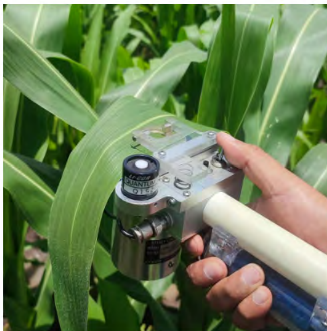
Figure 6. Clamp-type temperature measuring chamber of the LI-1600 porometer.
