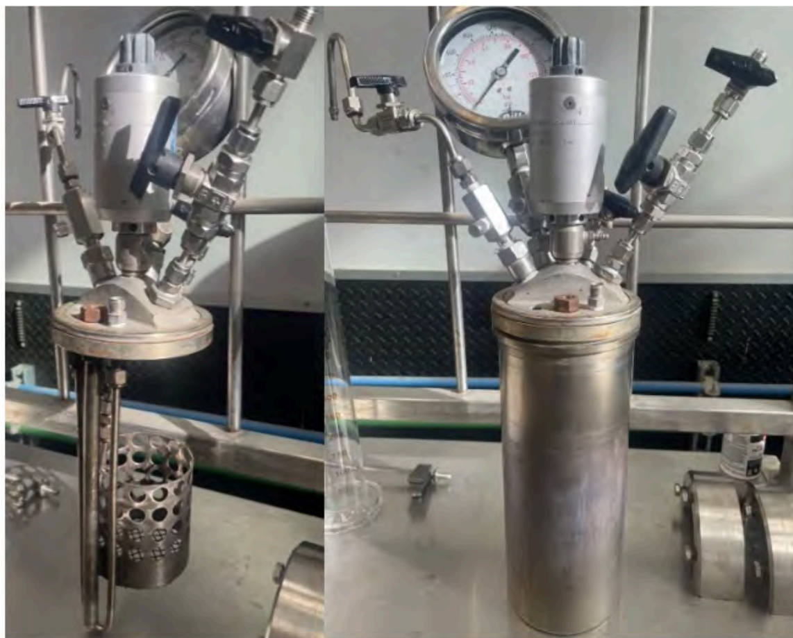
Figure 1. Reactor with a sample holder for the treatment of fibers by steam explosion.
