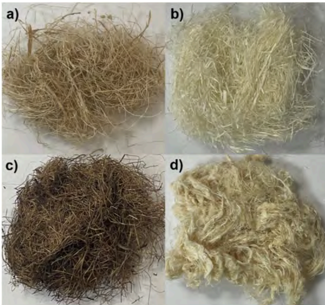
Figure 2. a) untreated banana fiber; b) NaClO-treated fiber; c) SE-treated fiber and d) fiber treated with SE and NaClO.
