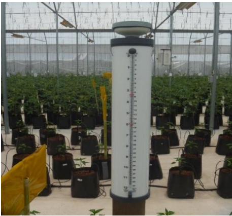
Figure 3. Installation of the atmometer inside the greenhouse.
