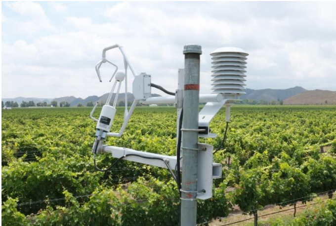
Figure 1. Sensors of an eddy system for measuring the flow of carbon dioxide between the canopy of the vineyard and the atmosphere. Production cycle 2018. Vinícola San Lorenzo, Parras, Coahuila, Mexico.
