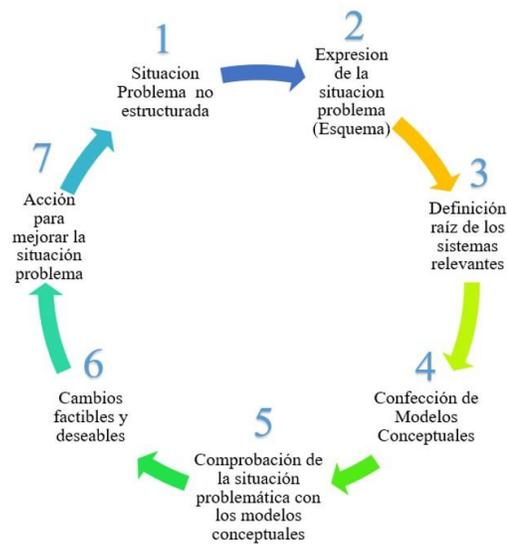
**Figure 1. Stages of the soft systems methodology (SSM) (Checkland and Poulter, 2006).**
