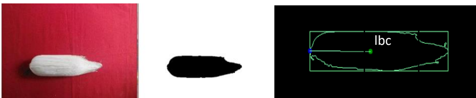
Figure 3. Processing of cobs in OpenCV to a) determine the area and b) lbc.
