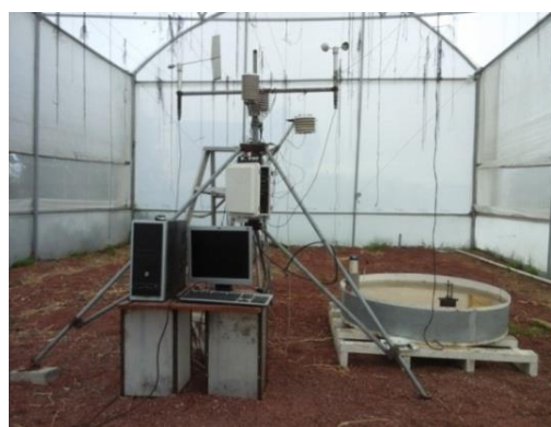
Figure 2. Automatic station inside the greenhouse.
