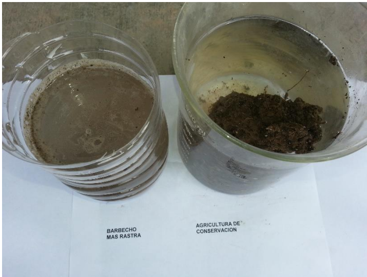
Figure 4. On the left, the B+R clod began to dissolve on contact with water, on the right, the clod with conservation agriculture was almost intact.
