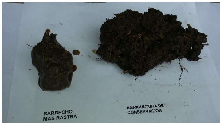
Figure 5. Size of the clods with B+R and conservation agriculture, after one minute of being submerged in water.
