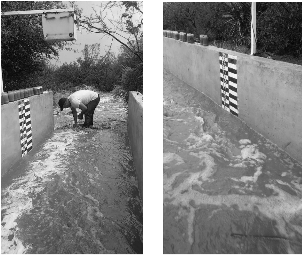
Figure 3. Sampling to determine the concentration of suspended solids in a runoff event during August 2016. INIFAP experimental basin, San Luis of Cordero, Durango.
