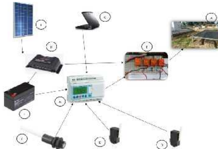
Figure 1. Scheme generating of the automatic control system: A) shadow mesh with motors; B) PLC; C) light sensor; D) position sensors; E) bridge H; F) batteries; G) laptop; I) solar panel; H) controller; and I) irrigation engine.
