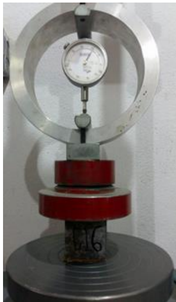
Figure 5. Resistance to compression in the GEOTEST press.
