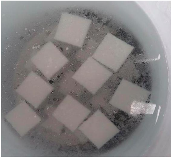
Figure 4. Curing of cubes.
