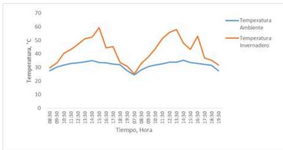
Figure 3. Comparison of ambient temperature with the interior temperature of the polycarbonate tunnel-type solar dryer in the Ranchería Miahuatlán, Cunduacán, Tabasco, Mexico using data Logger HOBO UX100-003.
