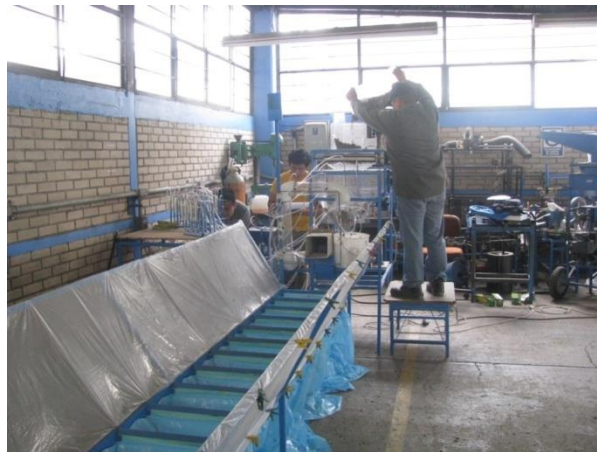
Figure 2. Test bench of the cleaning system and structure for the collection of the shell. Validation of air speed.
