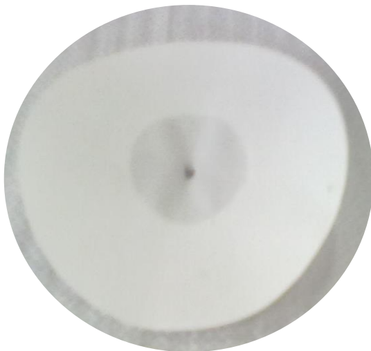
Figure 2. Number 1 Whatman filter paper impregnated with 0.5% silver nitrate.
